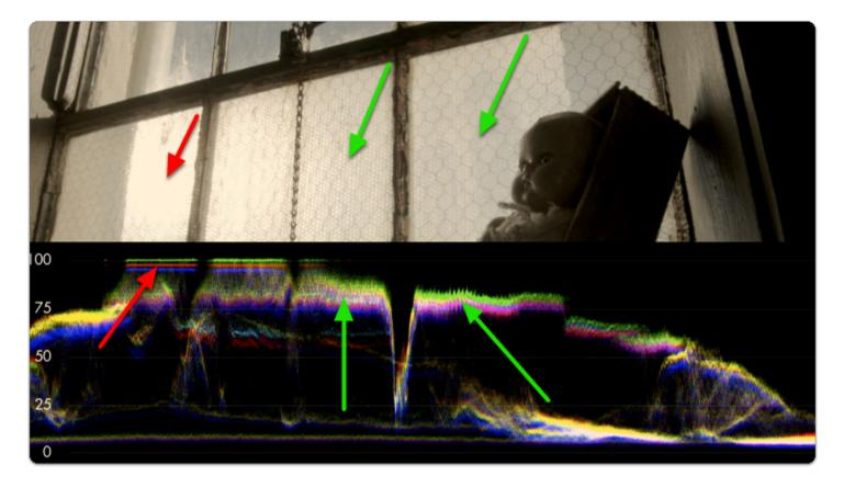
If we keep rolling exposure down (closing the aperture) we will continue seeing more 'into' the brighter details at the expense of **shadow details** which become '**crushed**' or '**clipped**' and **effectively lost** similar to overexposure.
