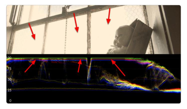
**Rolling exposure downwards**, the lines '**un-flatten**' and much more of the window can now be **manipulated in color grading** while some areas **remain overexposed**.
