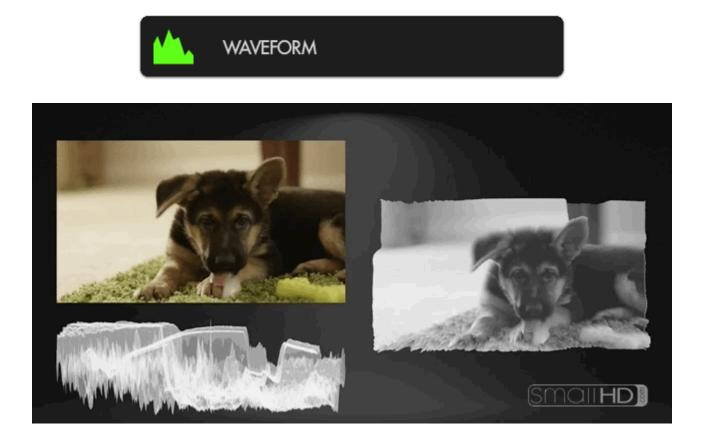
The **Waveform** is generally considered the **most robust exposure tool** because it plots your image's luminance (brightness) – and chrominance if using <u>RGB mode</u> – to a graph but unlike the Histogram, it physically **matches the screen from left-to-right**.
