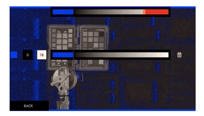
Set the **MIN** to **0** and adjust the **MAX** value to the point where color starts being introduced - You can customize this value until the **noise level** is acceptable to you (anything that gets painted blue is considered 'clipped', so increase the **MAX** to 'clip' more of the noise).
