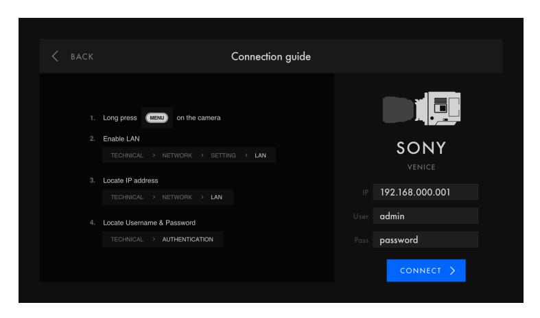
Connect an Ethernet cable to the Ethernet port on the monitor and on the camera. You can also connect to an Ethernet router as long as both the camera and monitor are visible on the same network.
