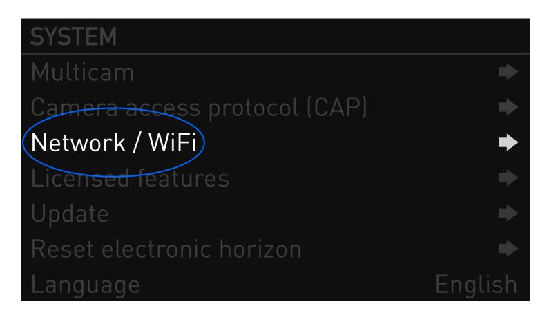
Press 'BACK' on the camera and navigate to 'Network / WiFi'
