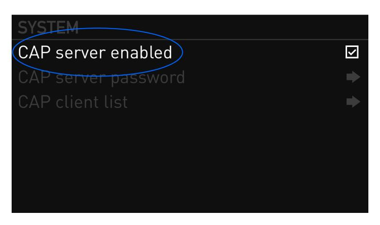
Ensure 'CAP server enabled' is checked—this is what will allow communication with the ARRI camera
