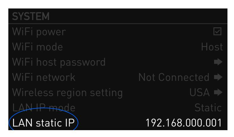
Lastly, make sure the IP Address field to the left matches the 'LAN static IP' field from the camera, then press Connect on your monitor
