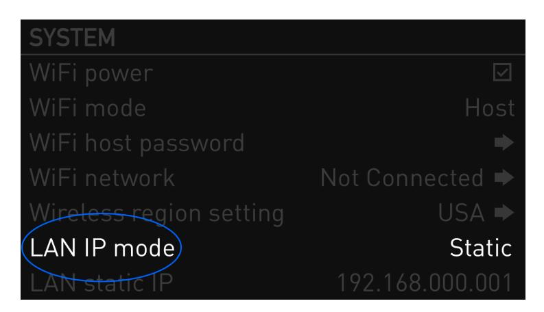
Ensure LAN IP mode is set to 'Static'
