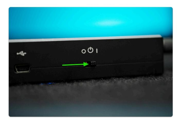
Using a **paperclip** (or similar precision instrument) press the **Reset** button on the transmitter until the **blue cloud LED** begins to **blink quickly**:
