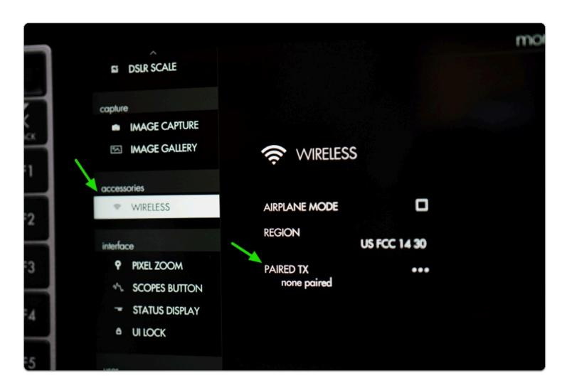
Click the joystick and select **PAIRED TX/RX** to enter pairing mode which will wait for a wireless signal from a <u>compatible transmitter(TX)</u> or Receiver (RX). Do this on both the TX and RX if you are pairing two SmallHD monitors.
