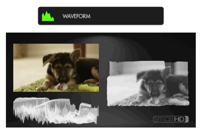
The **Waveform** is generally considered the **most robust exposure tool** because it plots your image's luminance (brightness) -- and chrominance if using <u>RGB mode</u> -- to a graph but unlike the Histogram, it physically **matches the screen from left-to-right**.
