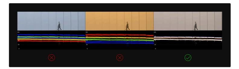
Notice how adjusting the white balance setting on the camera shifts the RGB 'bands' - when lined up they **turn white**, indicating a **proper white balance** setting.
