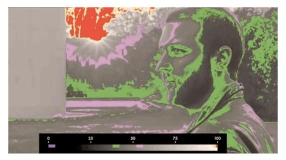
Exposure Assist is a **highly visible**, **quick** and **accurate** guide to setting exposure for your shots by 'painting' pixels when they hit a specified luma (brightness) value. This helps you **pinpoint** the exact areas your image may be **clipping** and quickly roll exposure to adjust for it, particularly in difficult viewing conditions (outdoors or on a gimbal or crane)
