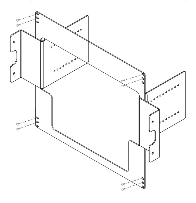
3. Slide monitor in between the Bracket Arms and attach with the four included thumbscrews
