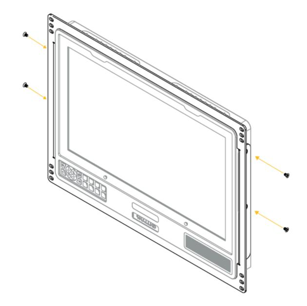
4. Attach the Rack Bracket to your rack system with the mounting screws that came with your rack system (these are not included, since they vary by manufacturer).
