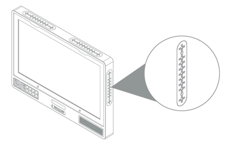
2. Insert monitor into Rack Bracket from the rear.
