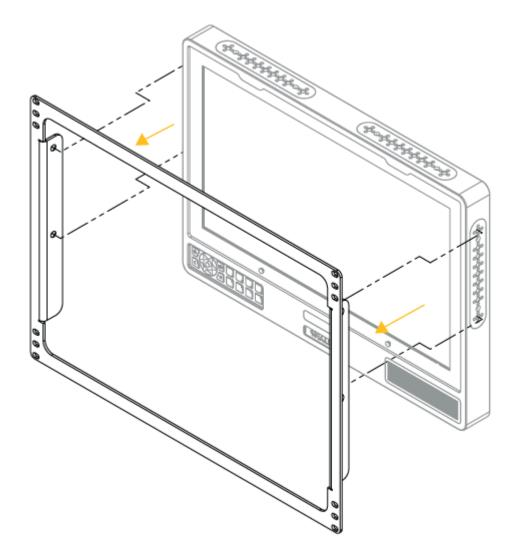
3. Attach the four screws (included) through the Rack Bracket into the Cheese Sticks on your monitor with a Phillips screwdriver.
