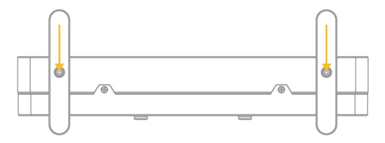
2. Attach the mounting rail to the bottom of the monitor using the captive screws already attached to the mounting rail.
