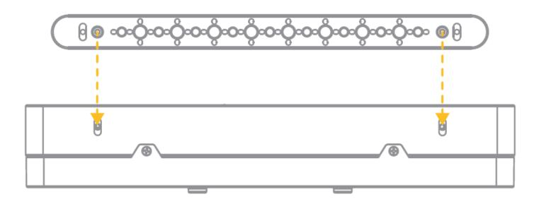
3. If desired, reattach the monitor feet to the mounting rail using a 3mm hex key and the two M4x10mm screws that were removed in step 1.
