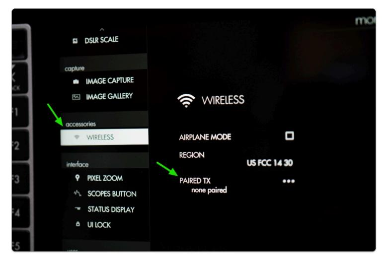
Click the joystick and select **PAIRED TX/RX** to enter pairing mode which will wait for a wireless signal from a <u>compatible transmitter</u>(TX) or Receiver (RX). Do this on both the TX and RX if you are pairing two SmallHD monitors.
