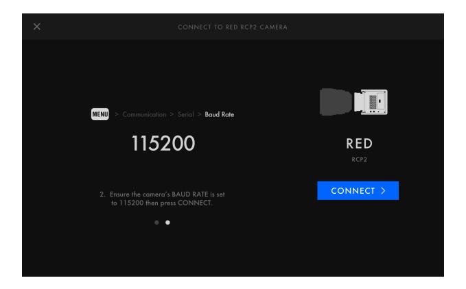
Connect your USB cable to the port on the back of your Monitor, wither directly using the Camera Control cable and USB adapter (If Applicable), below the battery plate. Tighten the locking connector into the adjacent screw for security. Connect the other end of the cable to your camera. Be sure the serial communication is enabled on the camera and that the baud rate is set to 115200.
